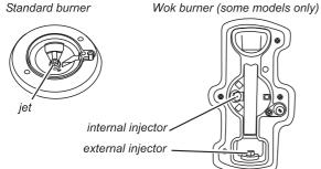
Remove burner caps and heads. Remove old jets. Fit the new jets (see **Technical Data** section at the back of the book for correct jets). Reassemble in reverse order.
